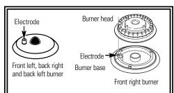
The electrode of the spark igniter is exposed when the burner head is removed. When one burner is turned to *LITE*, all the burners spark. Do not attempt to disassemble or clean around any burner while another burner is on. An electric shock may result, which could cause you to knock over hot cookware.
